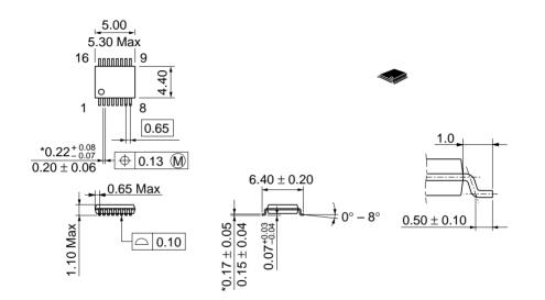
\*Dimension including the plating thickness Base material dimension
